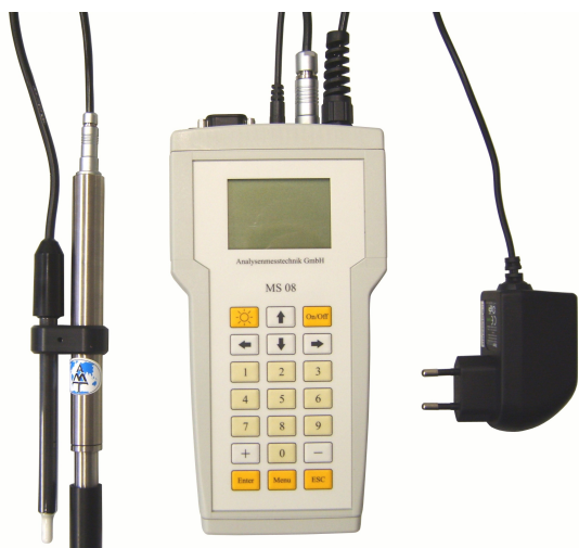
Fig.: Measuring Instrument MS 08 with micro-sensor, temperature sensor, RS 232 interface, power supply unit
